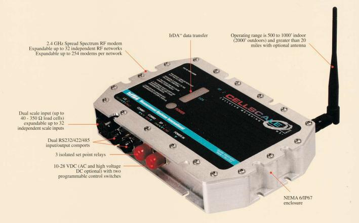
The MSI-9000 CellScale is the nucleus for a new and innovative approach to industrial weighing and process control ... called *Cellular Weighing*.
